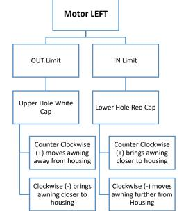
All negative (-) adjustments will only be noticed when the awning is under motion and comes to a stop. At that time, the awning will respond to positive (+) adjustments either towards the housing during IN limit or away from housing during OUT limit. **MOTOR MUST BE MOVING WHEN SETTING NEGATIVE (-) LIMITS**
